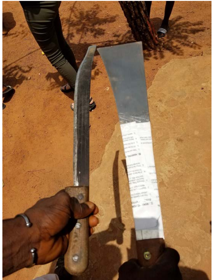
The labor-intensive nature of many of the cocoa-growing activities can be seen in how they wear down machetes, as displayed above. When it was new, the machete on the left was identical to the one on the right.
